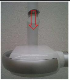
After removing the half-moon clip, pull down the tubehead to disassemble it.
