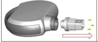
Once unscrewed the 3 fixing screws remove the internal part of the cone.
